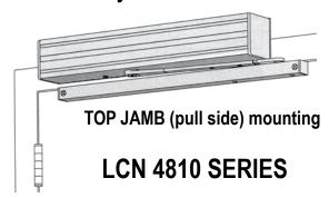
The 4810 AUTO-EQUALIZER™ is LCN's pneumatically powered MULTI-DOOR solution. This low-energy power operator provides easy access for people with disabilities, the elderly, or the frail. Designed primarily for manual opening applications that occasionally require automatic opening.
